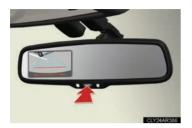
Press and hold the "AUTO" button for 12 to 15 seconds.
