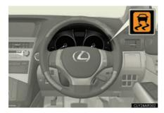
If the vehicle is in danger of slipping or if any of the drive wheels spins, the slip indicator light flashes to indicate that the VSC/TRC systems are operating.
