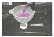
Add power control unit coolant if necessary.
