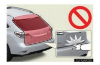
In the event that the back door is left slightly open, the back door closer will automatically close it to the fully closed position. It takes several seconds before the back door closer begins to operate. Be careful not to catch fingers or anything else in the back door, as this may cause bone fractures or other serious inturies.
