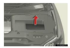
Removing the 12-volt battery cover.
