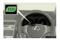
During Eco-friendly acceleration (Eco driving), Eco Driving Indicator Light will turn on. When the acceleration exceeds Zone of Eco driving, and when the vehicle is stopped, the light turns off.
