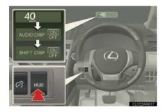
Press and hold the head-up display main switch changes the display to the display on/off mode. Press the head-up display main switch to select the desired setting item. Press and hold the head-up display main switch to turn the display on/ off.
