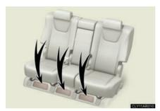
There are air intake vents under the rear seats for the purpose of cooling the hybrid battery (traction battery). If the vents become blocked, the hybrid battery may overheat, leading to a reduction in hybrid battery output.
