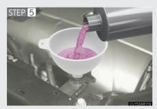
Add engine coolant if necessary.
