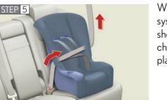
While pushing the child restraint system into the rear seat, allow the shoulder belt to retract until the child restraint system is securely in place.
