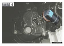
Replacing the light bulb, and install the bulb base.
