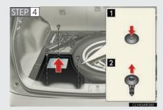
After removing the clips, remove the 12-volt battery cover.
