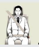
• Extend the shoulder belt so that it comes fully over the shoulder, but does not come into contact with the neck or slide off the shoulder.
