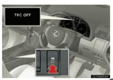
To turn the TRC system off, quickly press and release the switch.
