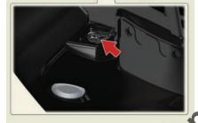
To allow enough working clearance, turn the steering wheel to the opposite side of the bulb to be replaced.
