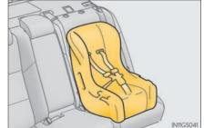
Run the seat belt through the child restraint system and insert the plate into the buckle.
