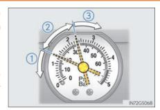
16 Turn the compressor switch on to inflate the tire until the recommended tire inflation pressure is reached. Drive for about 5 km (3 miles) and then perform step 14.
