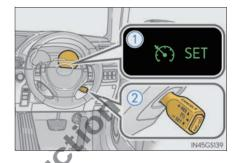
1 Press the "ON-OFF" button to activate the cruise control Cruise control indicator will come on. Press the button again to deactivate the cruise control.
